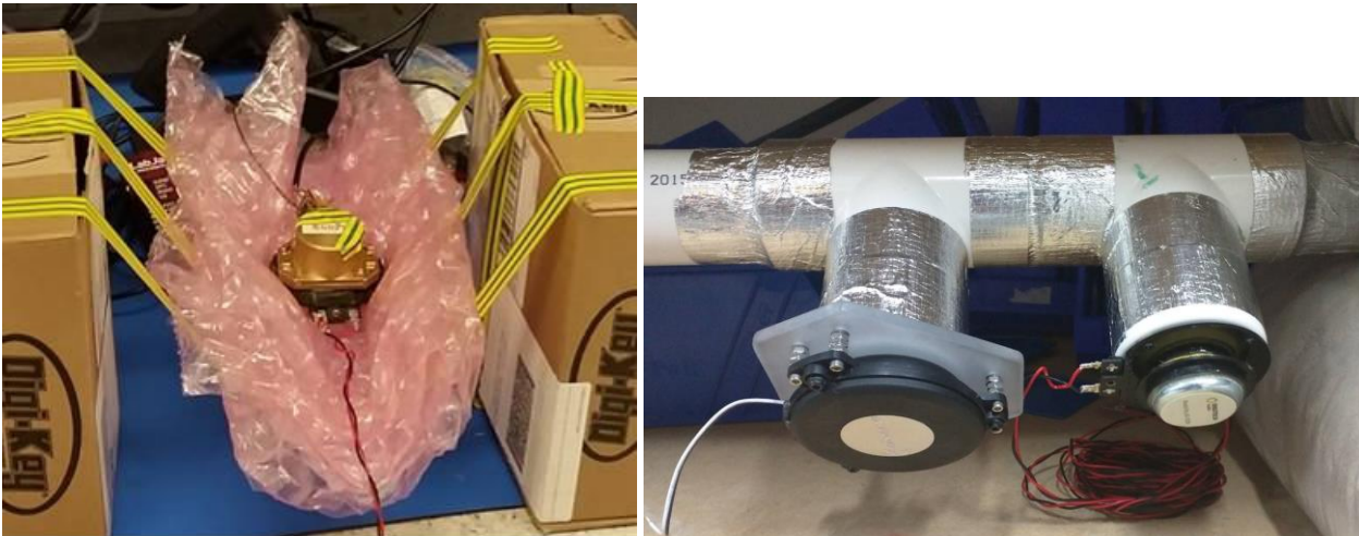
Figure 12 (left): background noise floor testing. Figure 13 (right): lab vibration test rig excitation diaphragms
