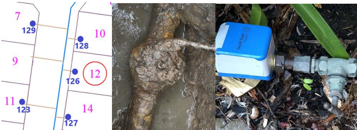
Figure 39 (left): water main and sensor GIS diagram. Figure 40 (middle): leaking service line connection. Figure 41 (right): leaking tail connection
